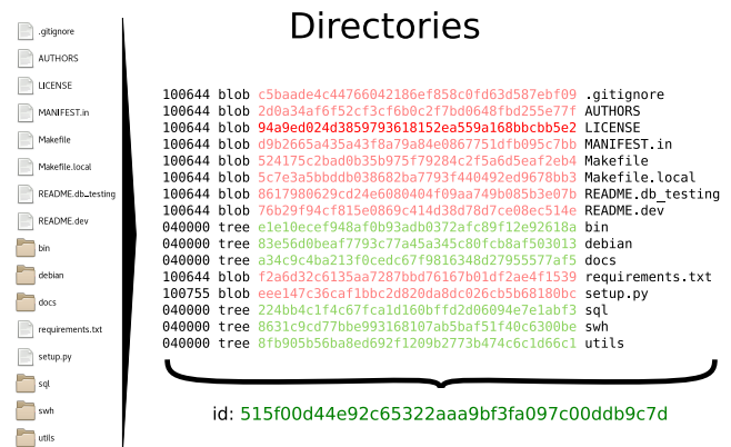
Fig. 2: Intrinsic identifiers in the Merkle DAG: example of how identifiers for directory nodes are computed.
